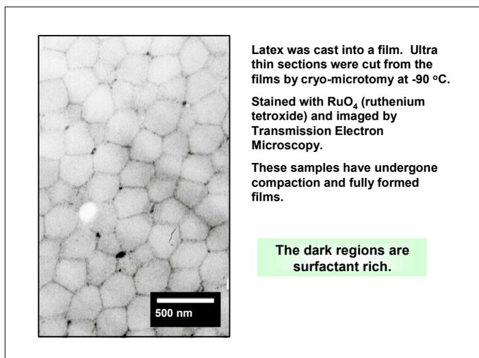
**Figure 1.** Transmission Electron Microscopy image of surfactant adsorbed at particle boundaries
