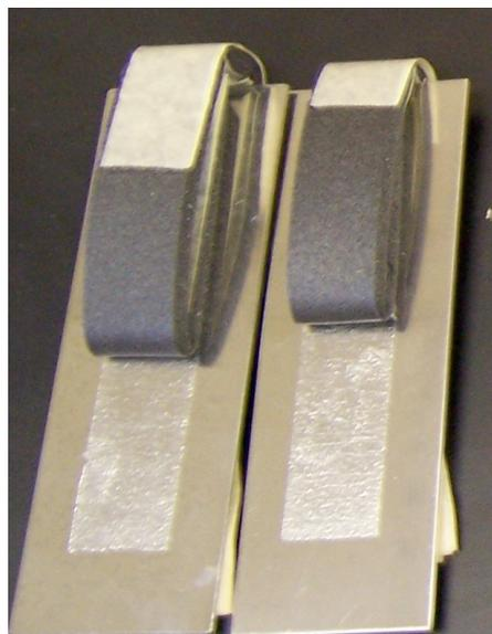
**Figure 4.** Adhesive failure to plasticized PVC foam with commercial aqueous PSA technology after automotive aging test (7days @70C)
