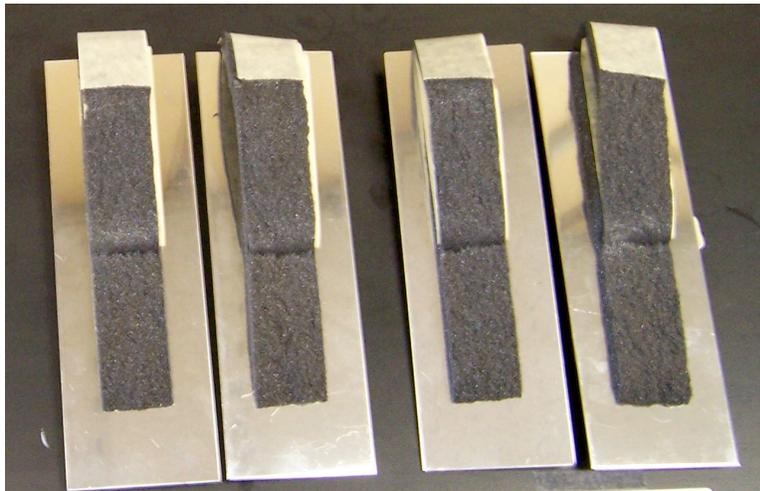
**Figure 3.** Plasticized PVC foam tear with modified emulsion PSA after automotive aging test (7days @70C)
