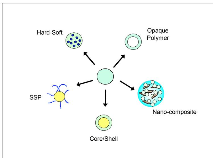
**Figure 2.** Acrylic polymer particle morphologies
